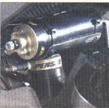
PENSKE rear shock has titanium spring
